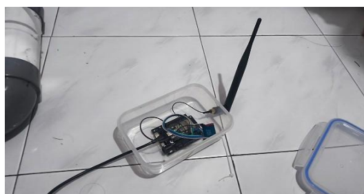
Gambar 6. Implementasi Node Receiver (Gateway)
