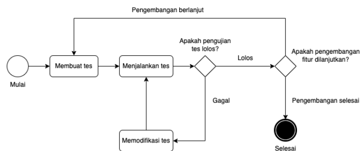
Gambar 2. Alur Metode Test Driven Development (TDD)
