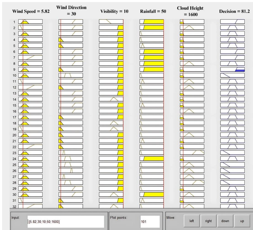
Figure 4. Fuzzy Testing Results. The decision output is 81.2% which indicates that the aircraft is not suitable for take-off/landing.
