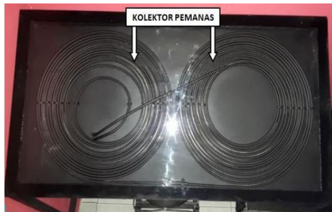
Gambar 3. Solar Water Heater Tampak Atas
