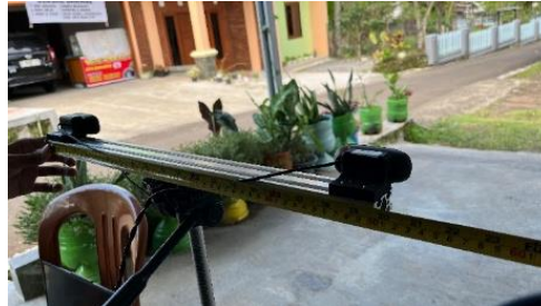
Figure 5. Stereo camera and luxmeter installation configuration
