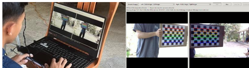
Figure 3. Stereo checkerboard detection results during calibration process
