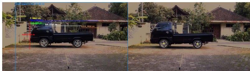
Figure 4. Real-time vehicle and wheel detection using YOLOv8 stereo vision system
